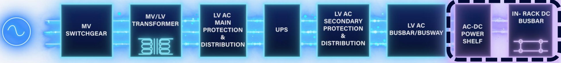
TODAY: OCP ORV3 ARCHITECTURE
