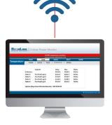
Temperature data also automatically transfer to the CPM's integral webpage—placing timely data at the end users fingertips.
