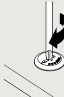
Drill a 14.1 mm hole in lid to accept turnbuckle
